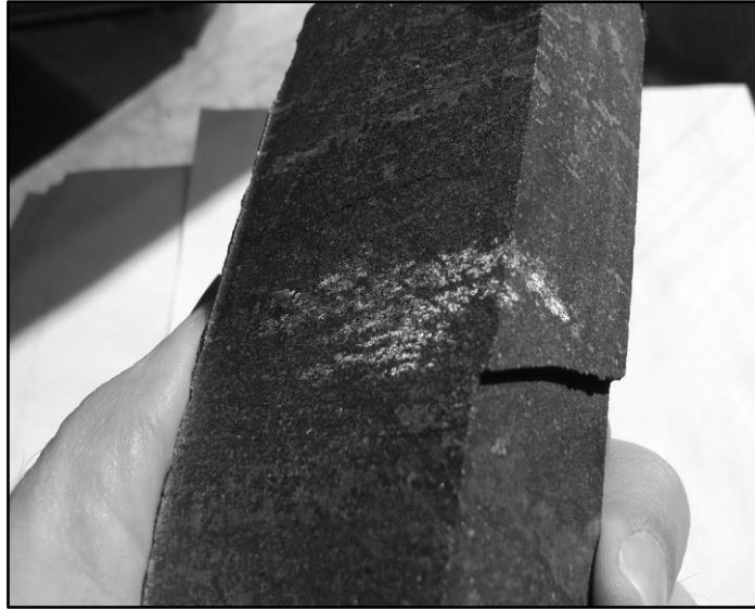
Figure 5. Cut slab of the Port Leyden nelsonite showing reflections from (0001) parting of single oikocrystic ilmenite grain (center). Slab width is 4 cm.
